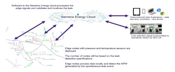
Figure 2. Siemens Energy SLD Service Architecture, powered by ProFlex Technologies
